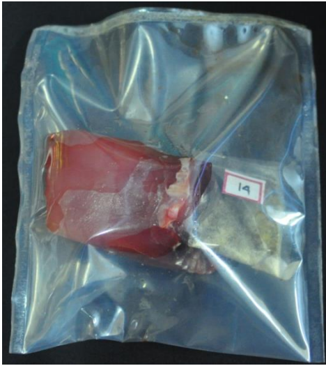
Plate 8.5 Yellowfin tuna chunk in EVOH pouch with developed dual action sachet SAIFC
