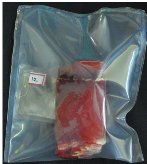
Plate 8.4 Yellowfin tuna chunk in EVOH pouch with developed dual action sachet SAI
