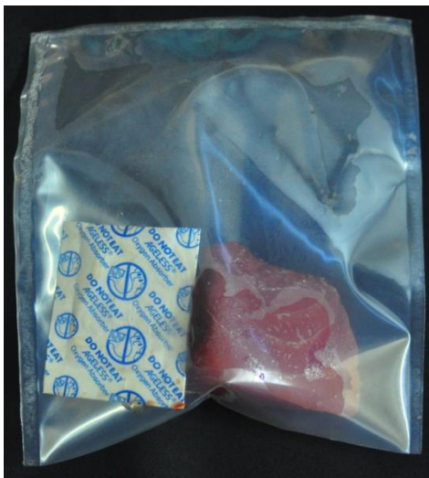
Plate 8.3 Yellowfin tuna chunk in EVOH pouch with commercial oxygen scavenger
