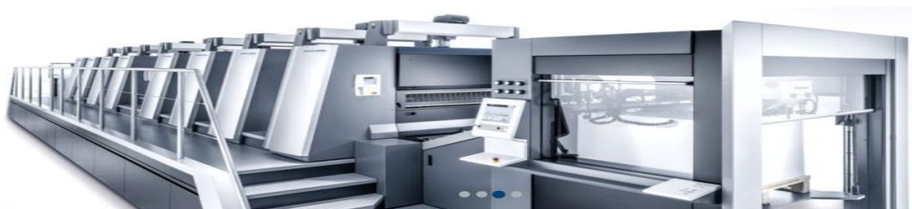
Fig. 3.3 Four Color Sheet fed Offset Printing Machine with perfecting (Heidelberg, Germany)
