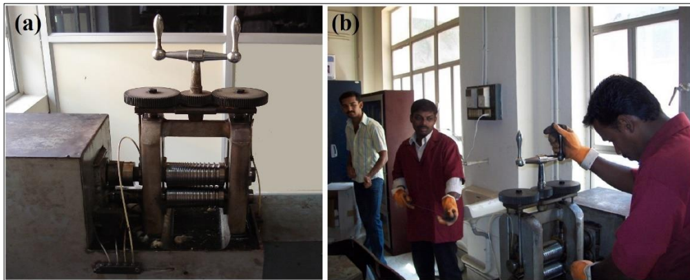
Fig (2.2) (a) Groove rolling machine, (b) Wire rolling in progress.
