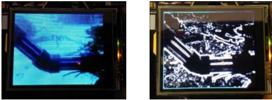
Fig. 6.5 Implementation of Edge Detection for a bent pipeline
