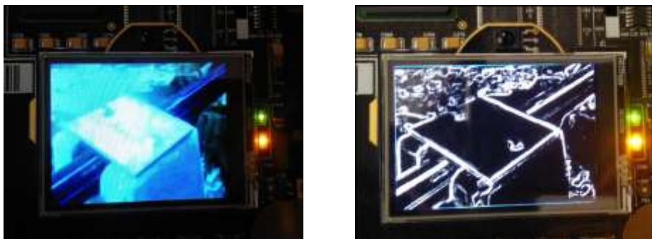
Fig. 6.6 Implementation of Edge detection for a partially submerged pipeline
