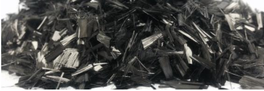
Figure 3.2 Photograph of short carbon fibers used for fabricating polymer FGM composites
