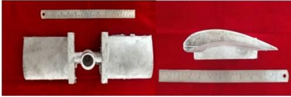
Figure 6.8 Photograph of the centrifugal cast functionally graded turbine exit vane guide
