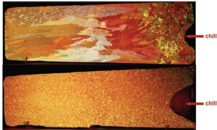
Figure 2.8 Grain structure in Al 3004 alloy (top: without grain refinement and bottom: with grain refiner 5Ti-1B alloy) (Geoffrey et al., 2007)
