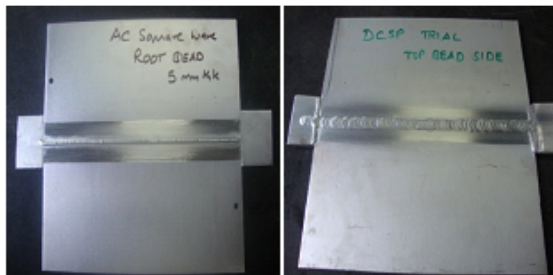
Figure 3.10: Samples of ACSQW and DCSP TIG welded joints
