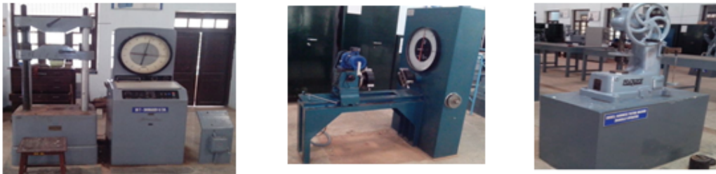
Figure 3.27: Machines used for tension, torsion and hardness tests
