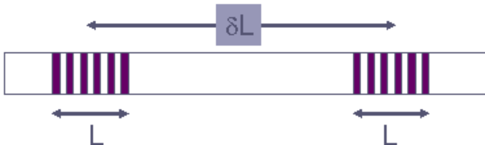
Fig. (2.14) Fabry-Perot filters using Fiber Bragg Gratings
