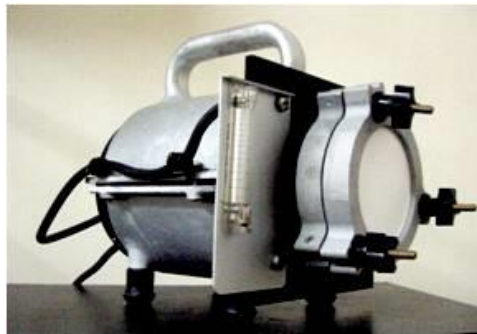
Figure 2.4. High Volume Sampler, model GH 2000 of Graseby Anderson.
