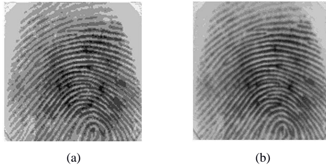
Figure 4.8 101_1.tif image reconstructed (with single-level, single training image, q = 64 ) using (a) classical (PSNR = 28.7516 dB, IE = 0.8114) , and (b) optimized (PSNR = 31.9427 dB, IE = 0.8117) wavelets.
