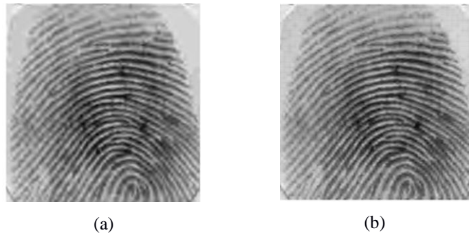
Figure 4.12 101_1.tif image reconstructed (with three-level MRA, three training images, q = 64 ) using (a) classical (PSNR = 31.6369 dB, IE = 0.2082), and (b) optimized (PSNR = 32.1426 dB, IE = 0.2150) coefficients.
