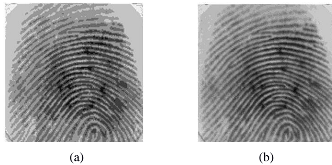
Figure 4.9 101_1.tif image reconstructed (with single-level, four training images, q = 64 ) using (a) classical (PSNR = 28.7516 dB, IE = 0.8114), and (b) optimized (PSNR = 32.0488 dB, IE = 0.8116) wavelets.
