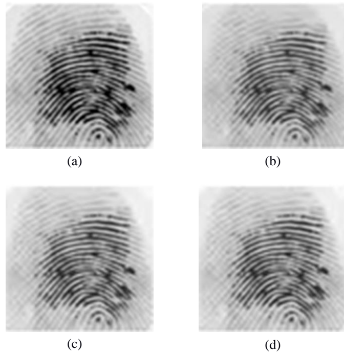
Figure 5.21 101_1.tif image (a) 15% degraded, Reconstructed with (b) classical wavelet (PSNR = 22.982 dB) (c) optimized coefficients from TIS_300 (PSNR = 23.088 dB) (d) optimized coefficients from TIS3_256 (PSNR = 23.056 dB).
