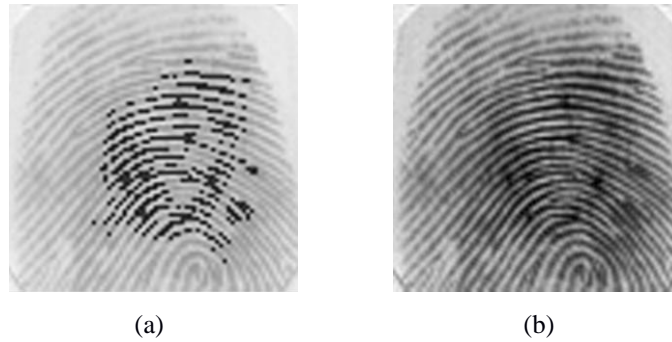
Figure 5.3 Reconstructed images after two-level transforms using (a) classical PSNR = 16.9083 dB (b) optimized coefficients (PSNR = 33.7334 dB), at CR = 16:1.
