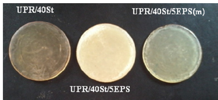
Fig. 7.5. Photographic images of the cured samples of synthesized resin samples at 40% styrene ratio
