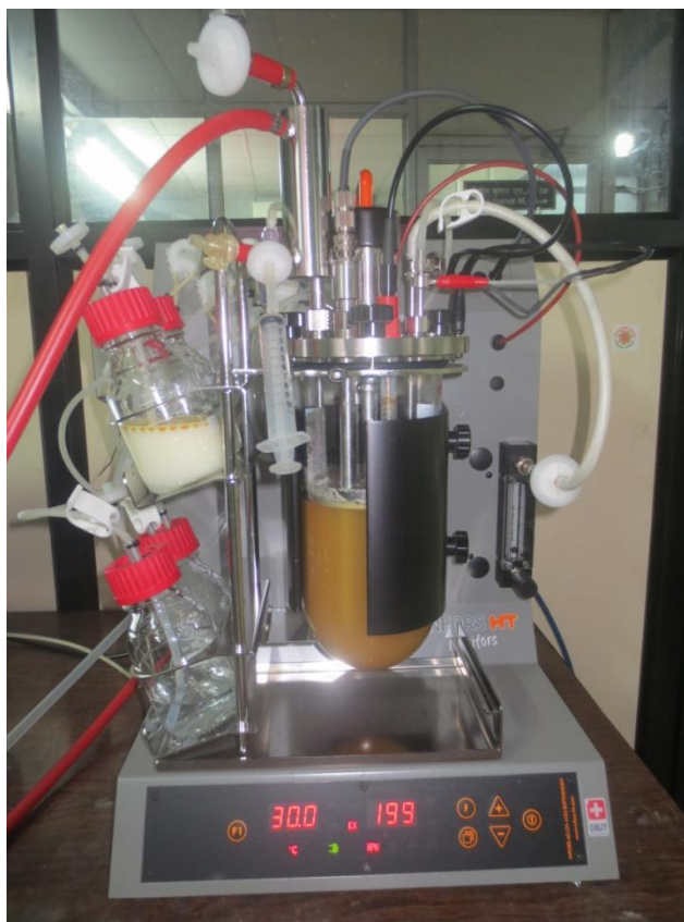
Fig 4.1. Experimental set up of 3L bioreactor for L-lysine production
