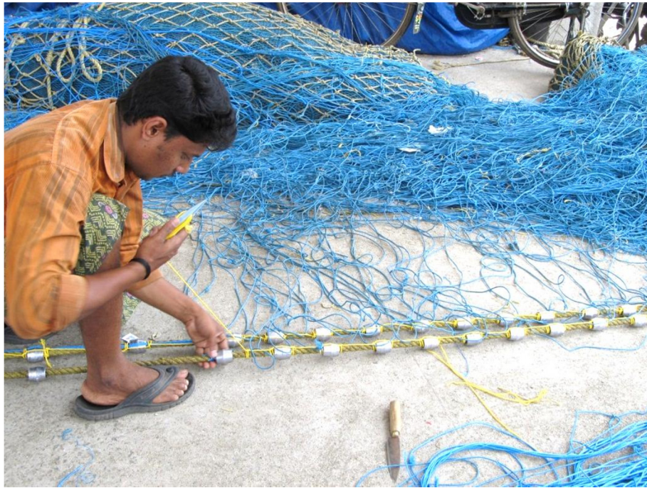
Fig. 5.4 Construction of a trawl net at Munambam
