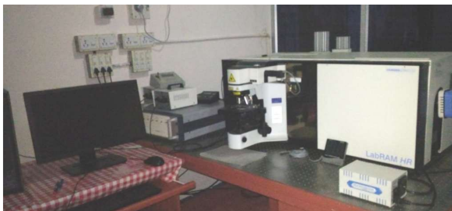
Figure 2.10. Horiba Jobin Yvon Lab Ram HR system used to record the Raman spectra of the samples under study.
