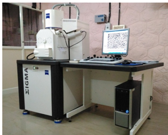
Figure 2.3. Carl Zeiss sigma field-emission scanning electron microscope (FE-SEM) used for the analysis of some of the samples under study.
