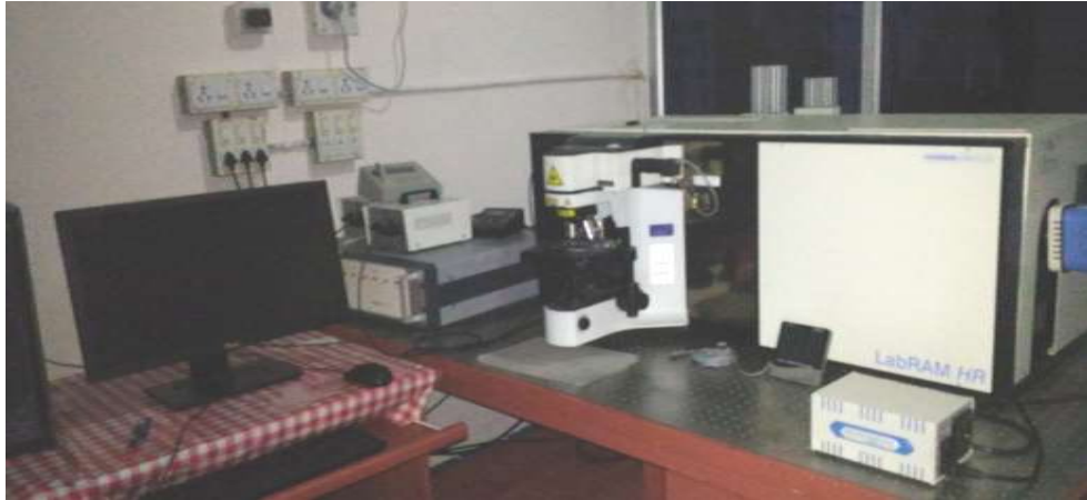
Figure 2.6. Horiba Jobin Yvon Lab Ram HR system used to record the photoluminescence spectra of the samples under study.
