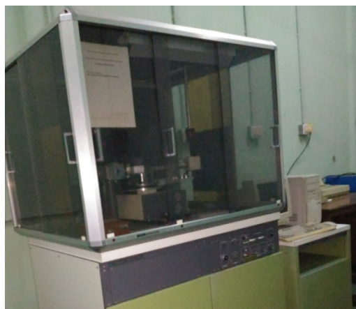
Figure 2.2. Rigaku Geigerflex D Max diffractometer with CuK \alpha radiation ( \lambda = 1.5414 \text{ \AA} ) used for the analysis of the samples under study.
