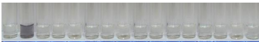
Figure 1.30 Visual color change of probe 38 ( 5.0 \times 10^{-5} M) with different cations: Sensor, \text{Hg}^{2+} , \text{K}^+ , \text{Na}^+ , \text{Ag}^+ , \text{Mn}^{2+} , \text{Ca}^{2+} , \text{Ba}^{2+} , \text{Fe}^{2+} , \text{Zn}^{2+} , \text{Pb}^{2+} , \text{Cu}^{2+} , \text{Sn}^{2+} , \text{Cd}^{2+} , \text{Ni}^{2+} and \text{Co}^{2+} ( 5.0 \times 10^{-5} M) 197
