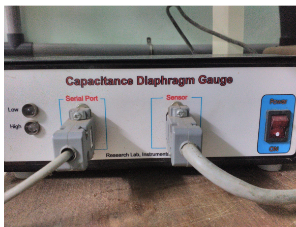
FIGURE 2.12: Photograph of the capacitance diaphragm gauge control unit.
