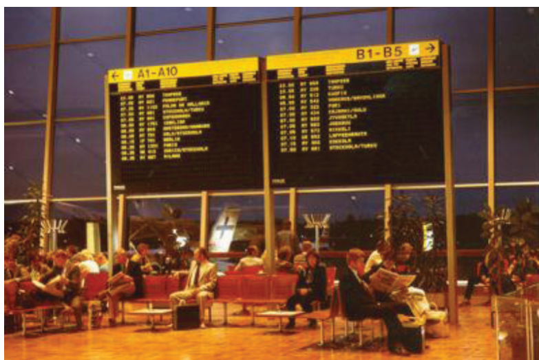
FIGURE 1.2: The first commercial application utilizing ALD: The flight information display by Lohja Corp. Display Electronics Division installed at Helsinki-Vantaa airport in 1983. [12]
