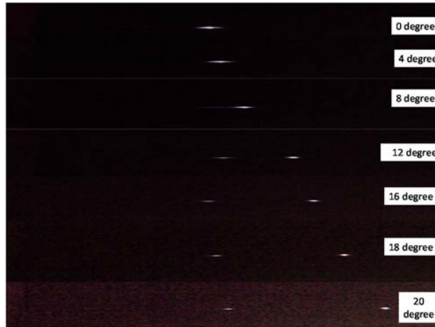
Figure 5.2: Filaments for different tilt angles under f/12 focusing geometry.
