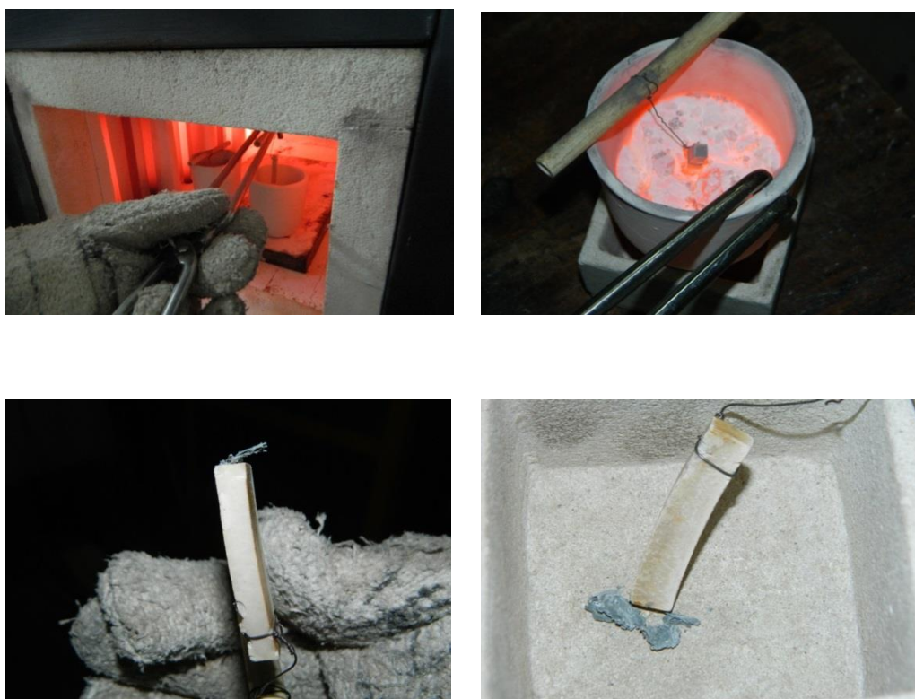
Figure 18) Photographs taken during the different steps of finger tests showing the metal chunks getting peeled easily of the surface
