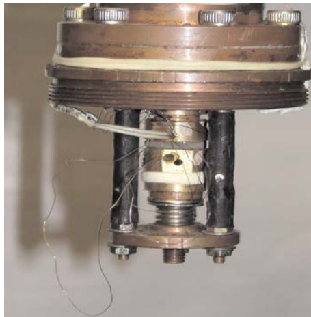
Figure 2.9: Photograph of the thermopower setup built on the cold head of a 4K CCR.
