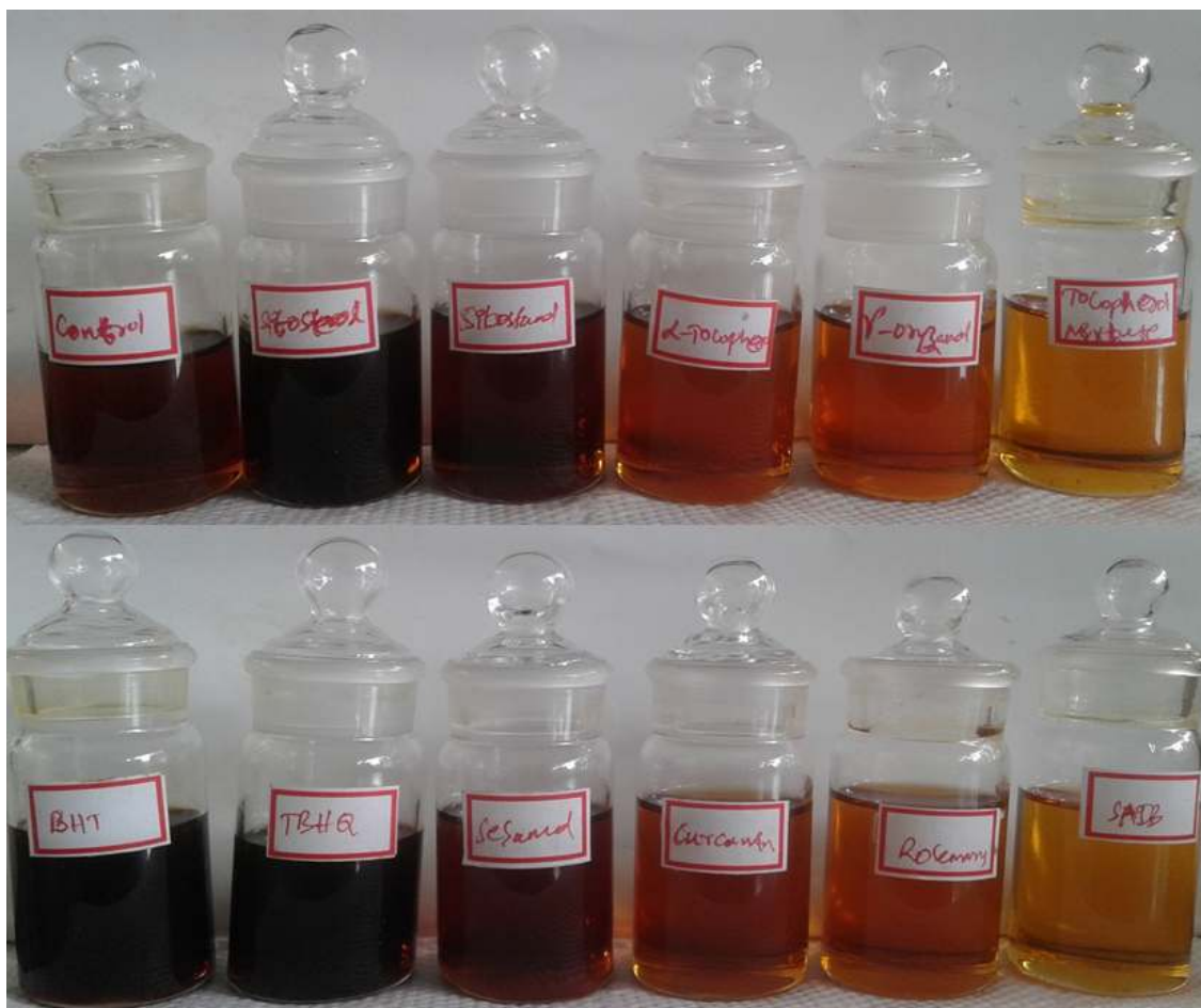
Figure 3.15 Physical appearance of soybean oil with different antioxidants after 6 hrs heating at frying temperature.
