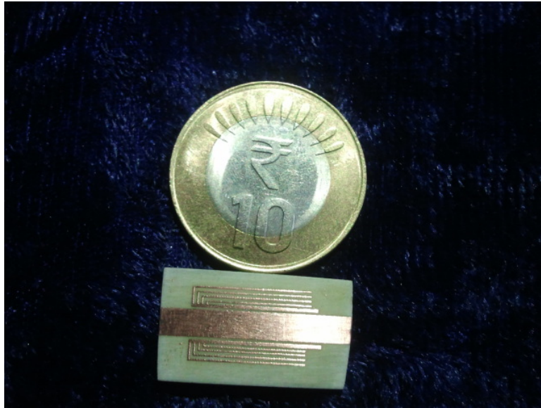
Figure 3.21: Photograph of the proposed multiresonator compared with INR 10 coin
