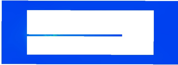
(b) Surface current distribution at non-resonant frequency (2 GHz)
