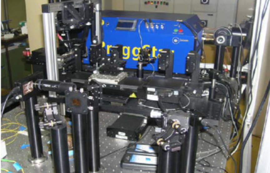
Figure 5.4: The grating fabrication setup used in CSIR- CGCRI, Kolkata.
