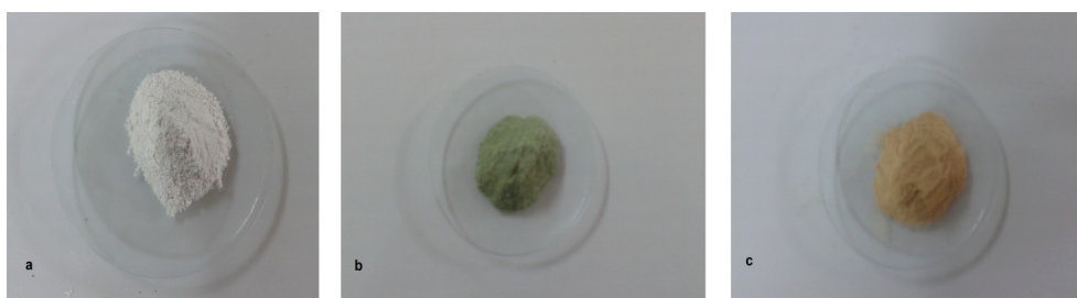
Fig. 3.4 \text{TiO}_2 obtained after calcination a) undoped \text{TiO}_2 b) Cu doped \text{TiO}_2 c) Fe doped \text{TiO}_2
