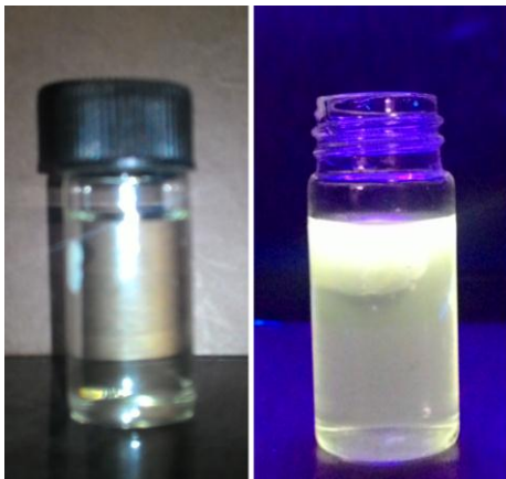
Figure 7:3 Photographs of TGA capped CdS QDs under visible light and UV light
