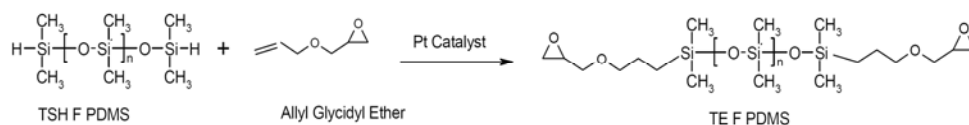
Scheme 2: Hydrosilylation of allyl glycidyl ether by terminal silyl hydride functional PDMS(TSHF PDMS)
