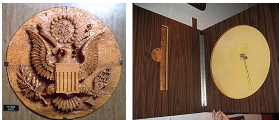
Figure 1.1 Great seal of United States and an exploded view of the device. Courtesy: Wikipedia.
