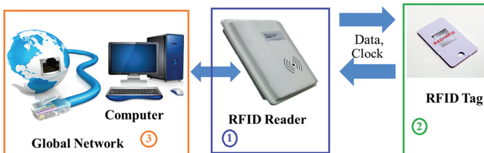
Figure 1.4 RFID System with three basic components, 1. RFID reader, 2. RFID tag and 3. Middleware software.
