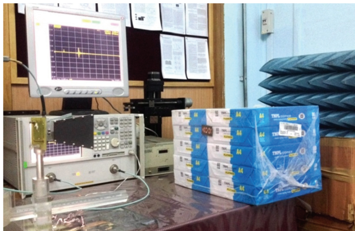
Figure 5.42 Measurement setup while placing RFID tag on a paper pack
