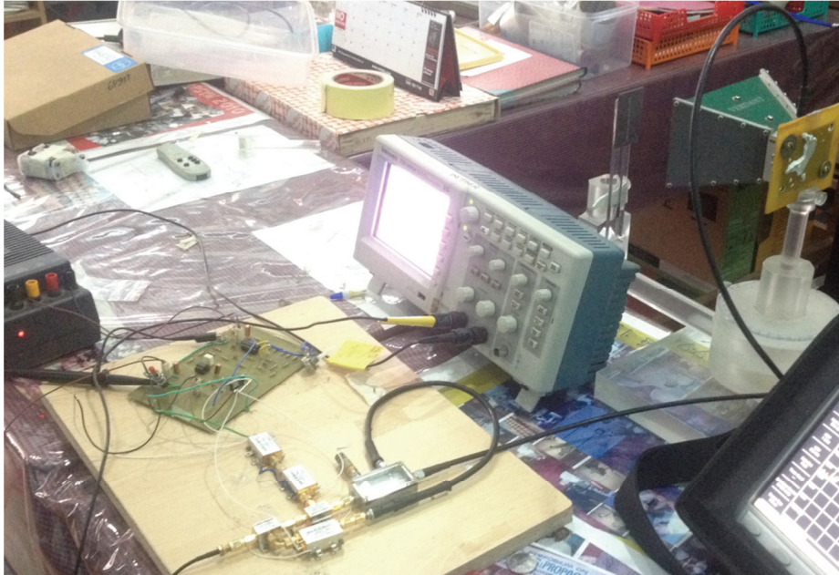
Figure 4.27 RFID reader measurement setup with an RFID tag placed at 5cm away from the antenna.
