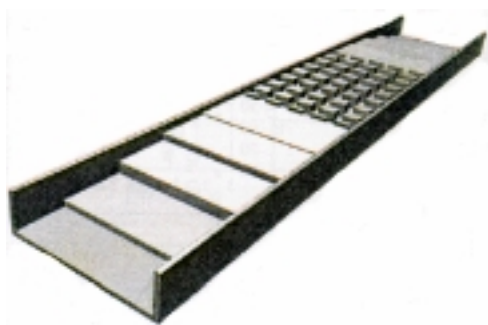
Fig (1). Half section of waffle-iron filter
