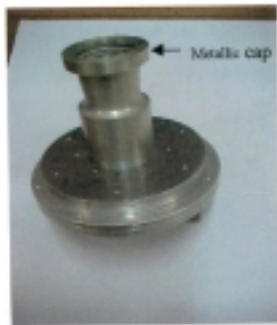
Fig 3. Monopulse multi mode horn along with planar comparator
