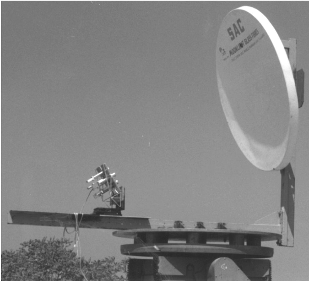
Fig. 1: Ku-band multiple spot-beam antenna on test range at SAC
