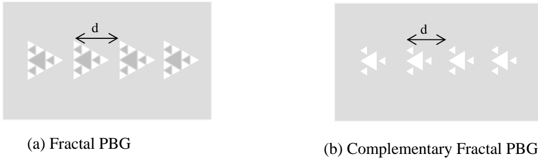
Fig.1: Geometry of the ground plane
