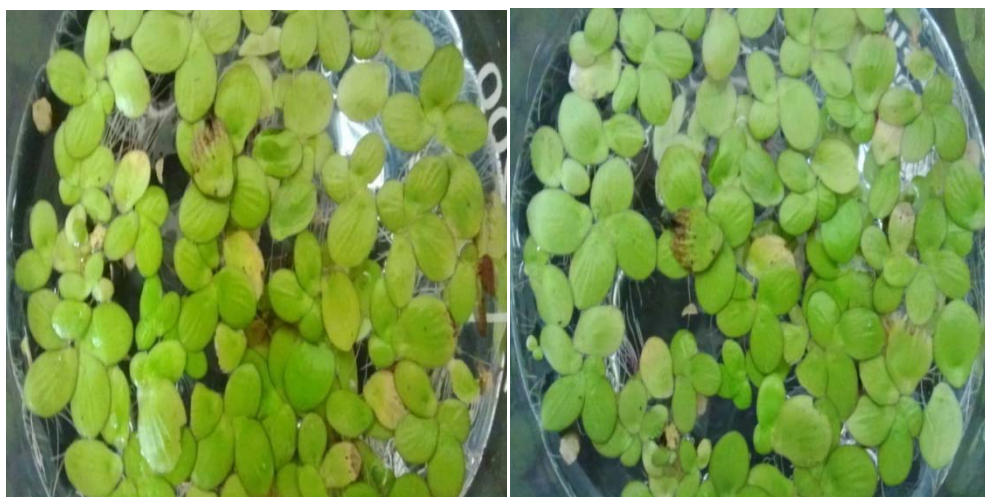
Fig.12(g): Comparison of Spirodela plant culture after 8 days of exposure in water sample from Kannamaly Wetland 1( left) and Wetland 2( right) during pre monsoon season. W1 sample exposure produces chlorosis on the fronds.
