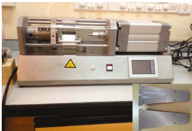
Figure 2.4 DSM Micro 10cc Injection Molding Machine
