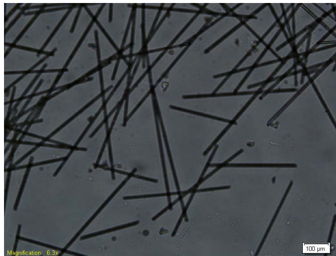
Figure 4b.2 Optical microscopic images of glass fiber for determining fiber length
