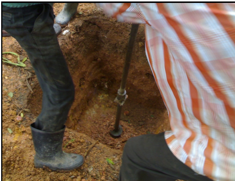
Fig. 3.4 Sample Collection using Hand Auger
