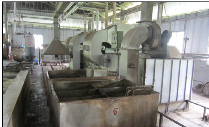
Figure1.7 View of crumb drier
