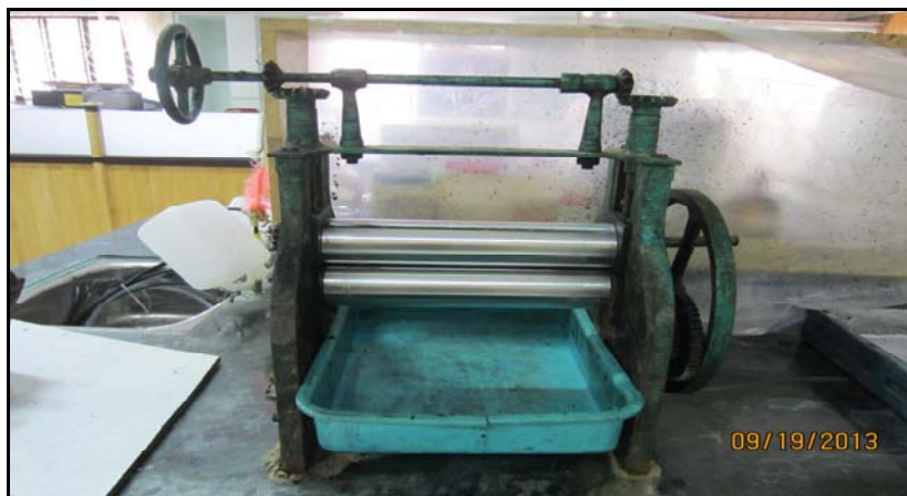
Figure 2.4 Roller for sheeting coagulum.
