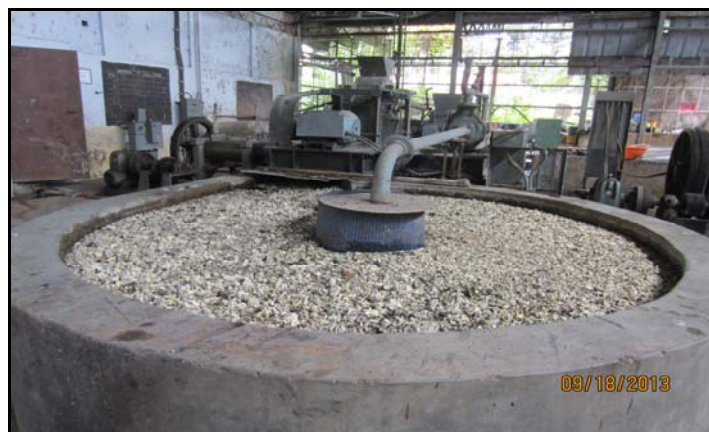
Figure 1.5 Crumbs collection tank
