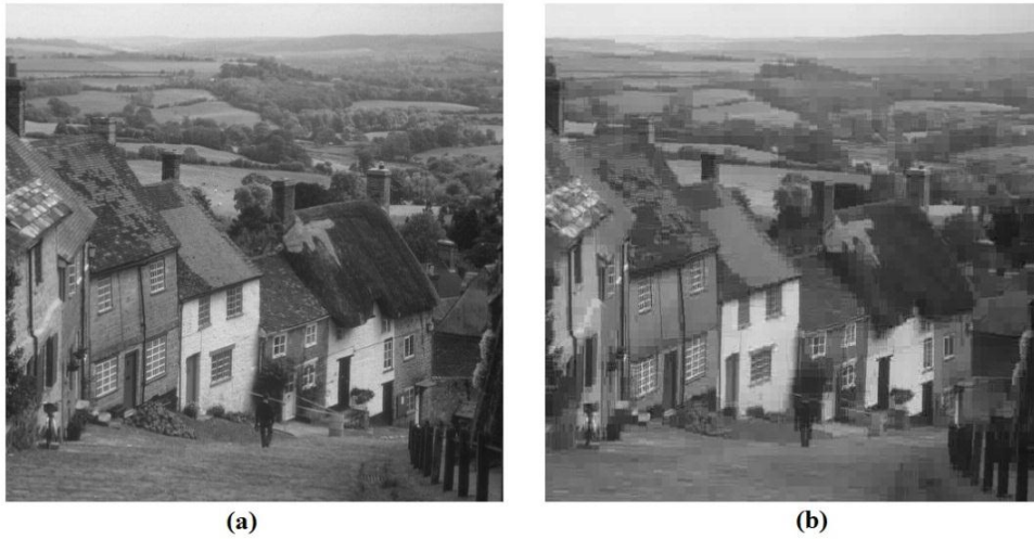
Figure 3.19: Goldhill (512×512) (a) original and (b) reconstructed after compressed using 8×8 MRT based transform coder (threshold 150, bpp 0.50, PSNR 29.09)
