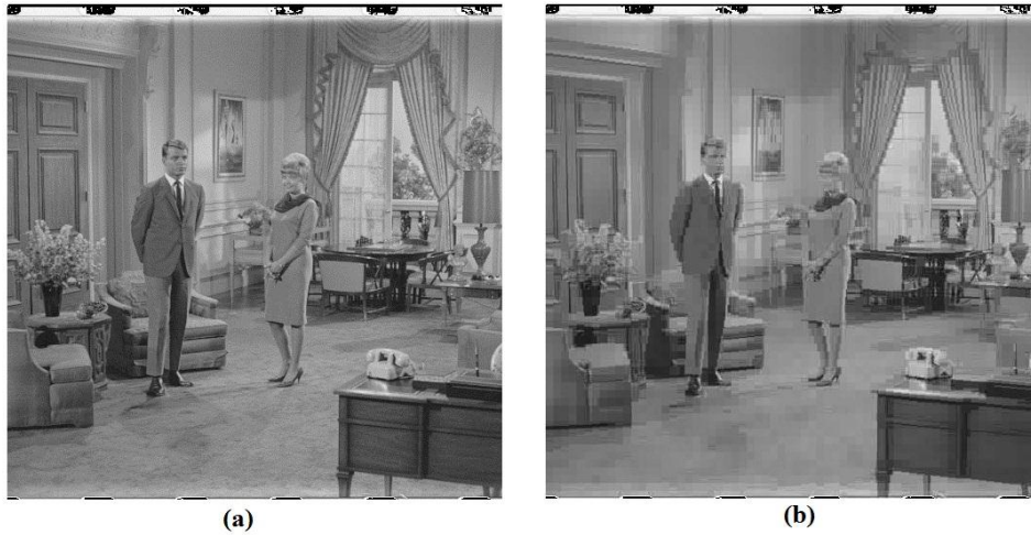
Figure 3.17: Couple (512×512) (a) original and (b) reconstructed after compressed using 8×8 MRT based transform coder (threshold 150, bpp 0.63 , PSNR 30.11)
