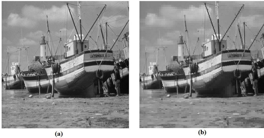
Figure 3.15: Boat (512×512) (a) original and (b) reconstructed after compressed using 8×8 MRT based transform coder (threshold 150, bpp 0.63, PSNR 28.89)
