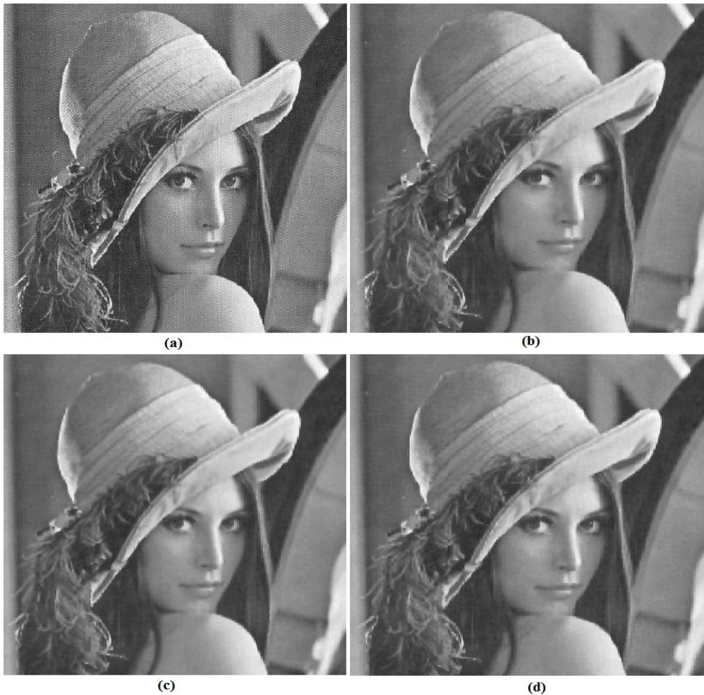
Figure 4.2: (a) Original Lena (512×512) image (b) – (d) reconstructed versions after compressed at 0.30 bpp using hybrid coder, 8 \times 8 MRT based transform coder and 4 \times 4 MRT based transform coder respectively.
