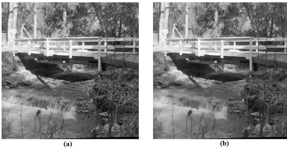
Figure 3.16: Bridge and stream (512×512) (a) original and (b) reconstructed after compressed using 8×8 MRT based transform coder (threshold 150, bpp 1.01, PSNR 26.29)
