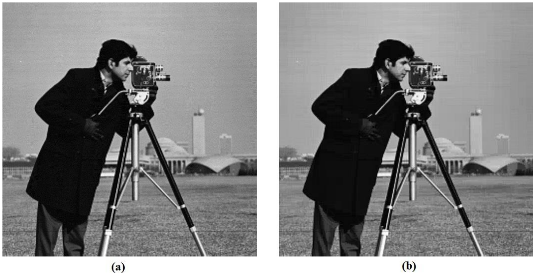
Figure 5.20: Cameraman (a) Original and (b) reconstructed after compressed using MATC-CVQ coder (bpp =0.430, PSNR = 33.25).
