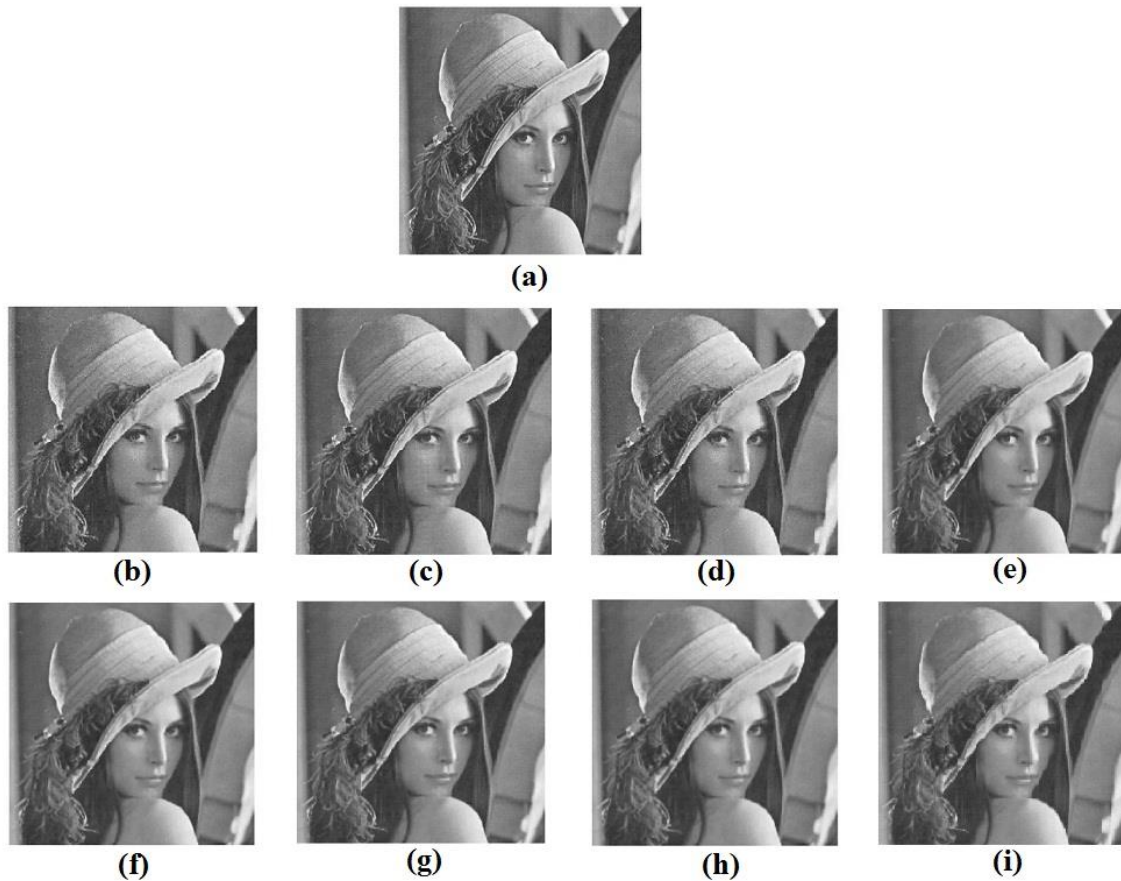
Figure 3.25: Lena (512×512) (a) original and (b) – (i) reconstructed after compressed using 4×4 MRT based transform coder with bpp 0.91, 0.58, 0.44, 0.38, 0.34, 0.32, 0.31 and 0.30 respectively
