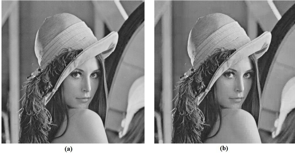
Figure 5.18: Lena (a) Original and (b) reconstructed after compressed using MATC-CVQ coder (bpp = 0.33, PSNR = 32.89 )
