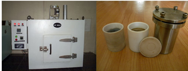
Figure 2.2: Hydrothermal furnace and autoclave used for the synthesis of nanostructures.
