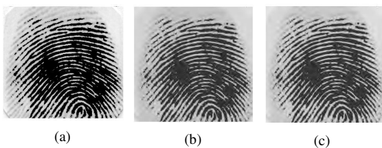
Figure 7. 101_1.tif image (a) with 40 % degradation (b) reconstructed image using theoretical coefficients (c) reconstructed image using evolved coefficients.
