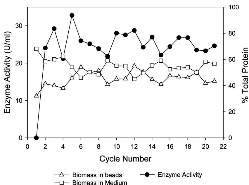
Fig. 1. Repeated batch production of L-glutaminase by Ca-alginate immobilized cells.
