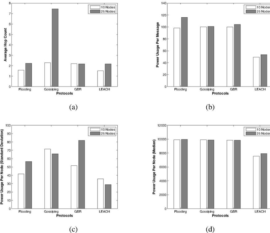
**Fig. 1:** Results of simulation (a) Average hop count of the messages forwarded by the base station. (b) Power usage per message sent. (c) Power usage per node (Standard Deviation). (d) Power usage per node (Median).
