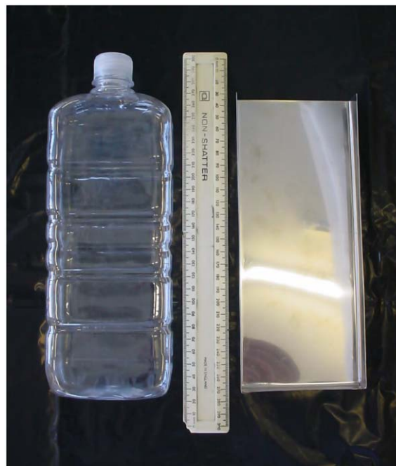
Fig. 1 – Photograph of custom-made solar disinfection reactor, 48 g PET (left) and stainless steel reflector (right) alongside a 30 cm ruler, for scale.
