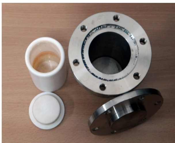
Figure 2.1 Autoclave and container used for the synthesis of FeS 2 /polymer nanocomposites
