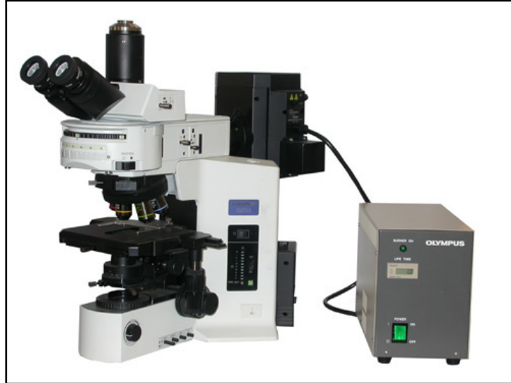
Figure 2.9 The Olympus BX51 Fluorescence Microscope
