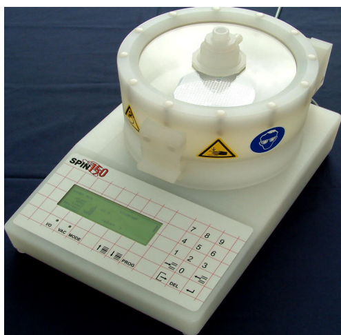
Figure 2.2 Spin-coating unit (Spin 150)
