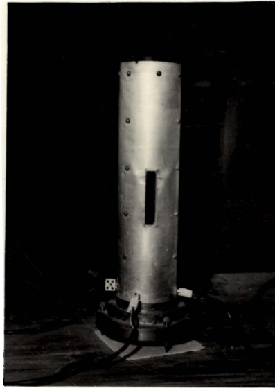
Fig.2.2 Photograph of the furnace used for growing crystals from melt.
