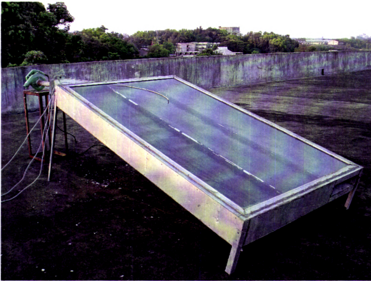
Fig. 3.12 Experimental set up on copper collector
