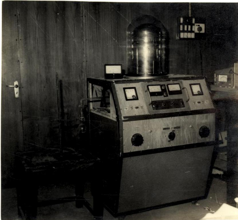
Fig.2.64 The plasma-polymerisation chamber
