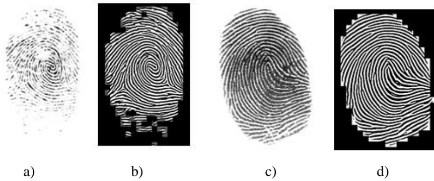
Fig. 4.7 a) and c) Fingerprint images and b) and d) Gabor filter based enhanced images
