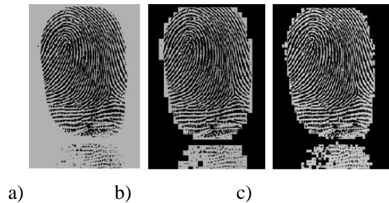
Fig.3.6 a) Fingerprint image b) Segmented image with w = 16 c) Segmented image with w = 8
