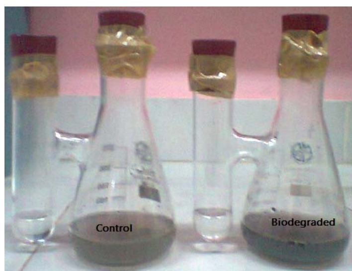
Fig.4.69 Biodegradation of asphaltene by L.fusiformis BTTS10 in biometric flasks
