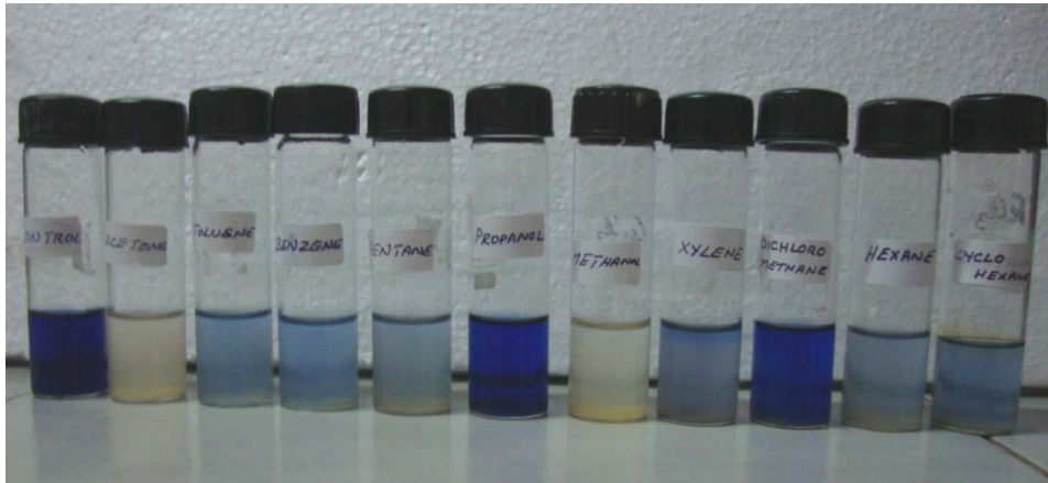
Fig. 4.13. Use of DCPIP as an indicator of biodegradation of hydrocarbons by L.fusiformis BTTS10
