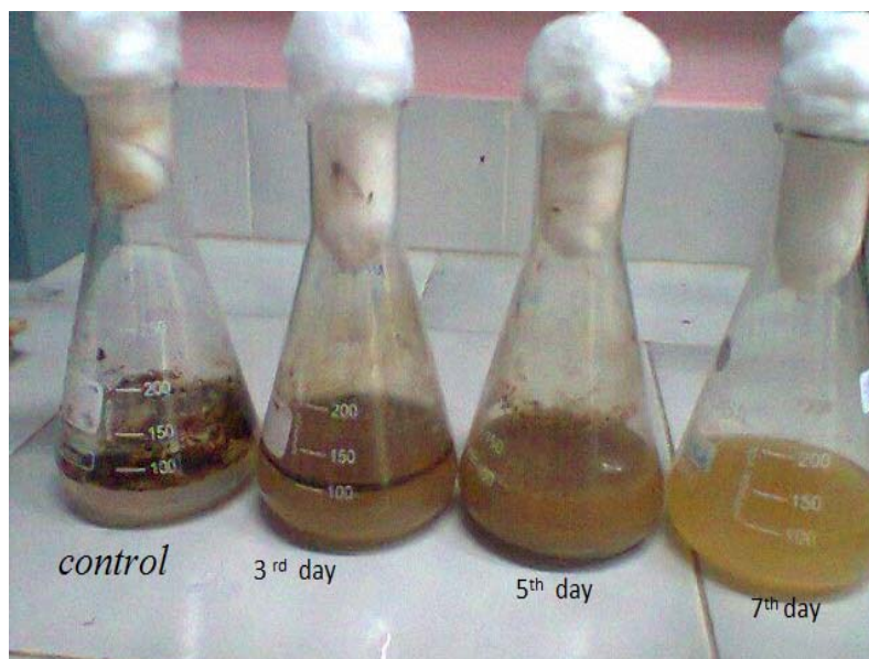
Fig.4.17 Macroscopic view of biodegradation of crude oil by L.fusiformis BTTS10
