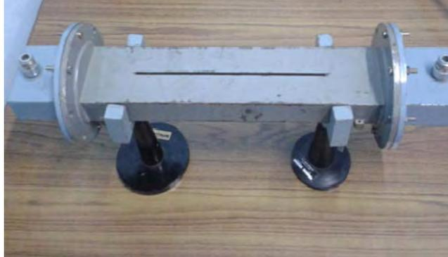
**Fig. 2.3** The S band wave-guide cavity resonator
