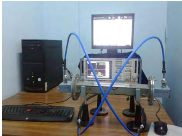
**Fig. 2.4** Setup for the measurement of microwave properties
