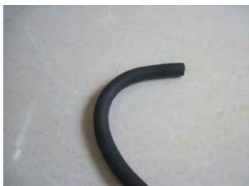
**Fig. 8A.2 Expanded EPDM ( $E_{mix}$ ) extruded sample**
