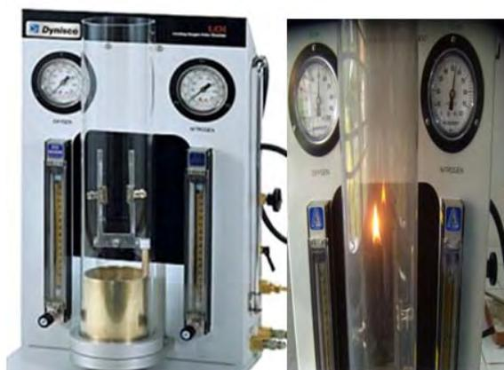
**Fig. 7.32 Photograph showing sample testing procedure in an LOI instrument**
