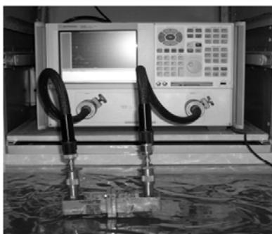
**Fig. 2.5 Set-up for EMI shielding measurement**
