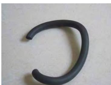
**Fig. 8A.3 Expanded EPDM/Viton blend ( $EV_{mix}$ , 80:20) extruded sample**
