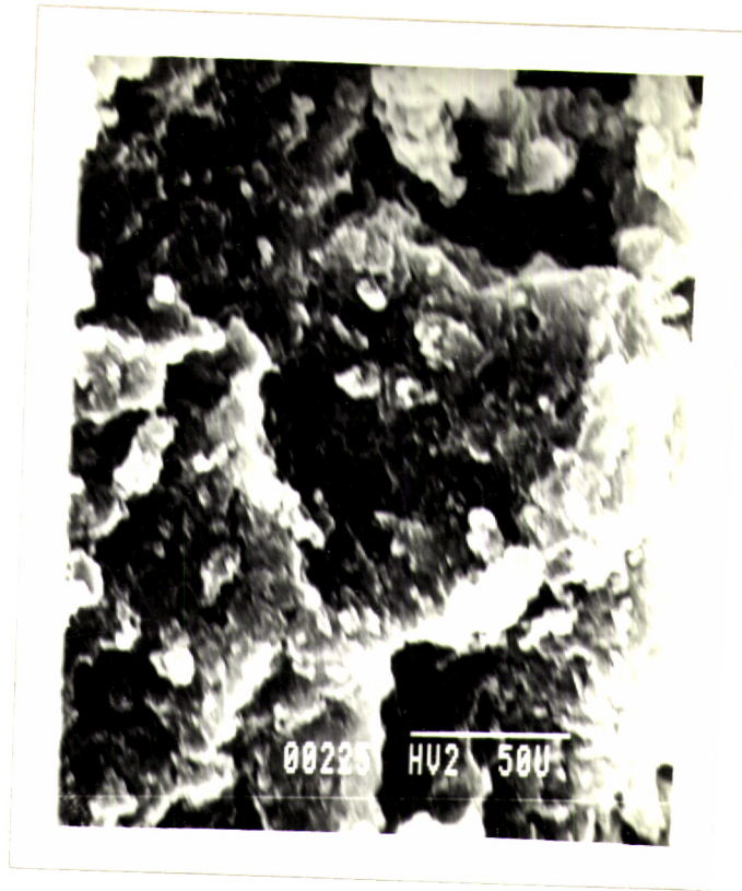
Fig.4.37 SEM Photograph of abraded surface of 100% LR(T) vulcanizate
