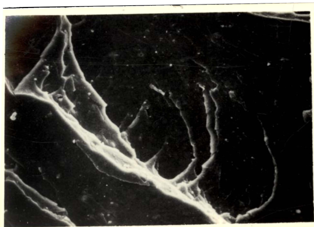
Fig.7.5 Tensile fracture surface of vulcanizate 5 (Table 7.2)
