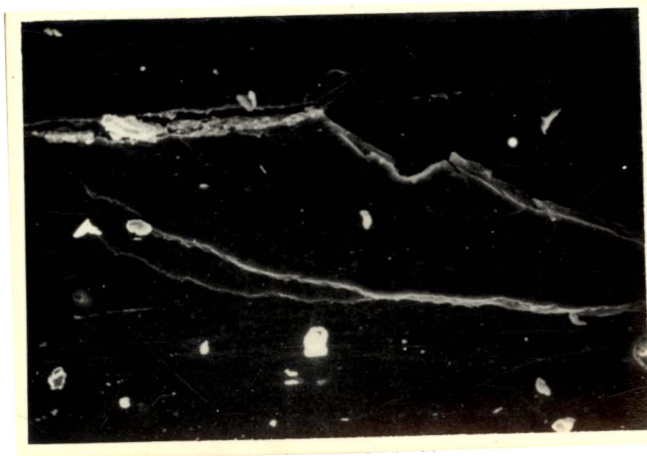
Fig.7.17 Tensile fracture surface of vulcanizate 9 (Table 7.3)
