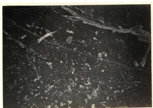
Fig.7.19 Tensile fracture surface of vulcanizate 11 (Table 7.3)
