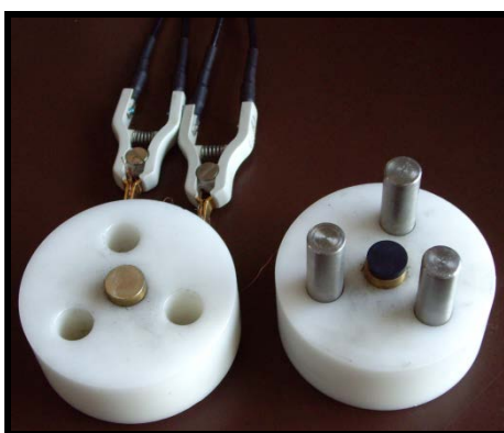
Figure 3.5(a): Sample holder used in the experiment to measure the change in conductivity with applied load using 2-probe method
