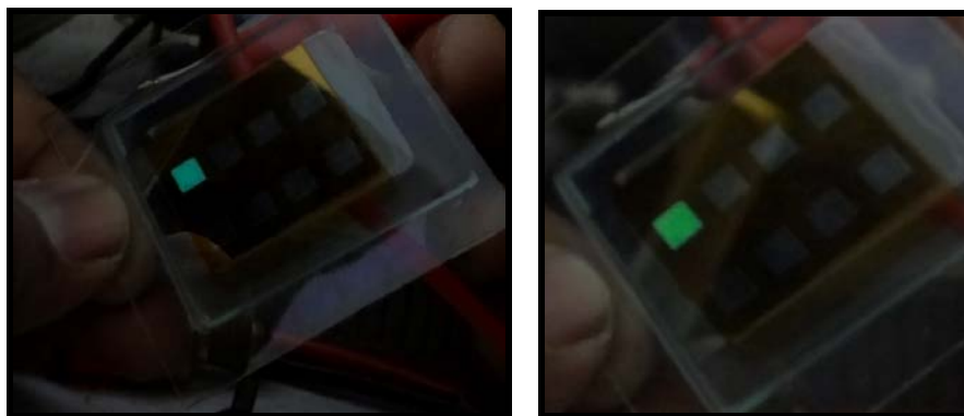
Figure 7.13: Electroluminescence emission from the prototype devices fabricated using (a) P1 (blue-green) and (b) P2 (green) respectively
