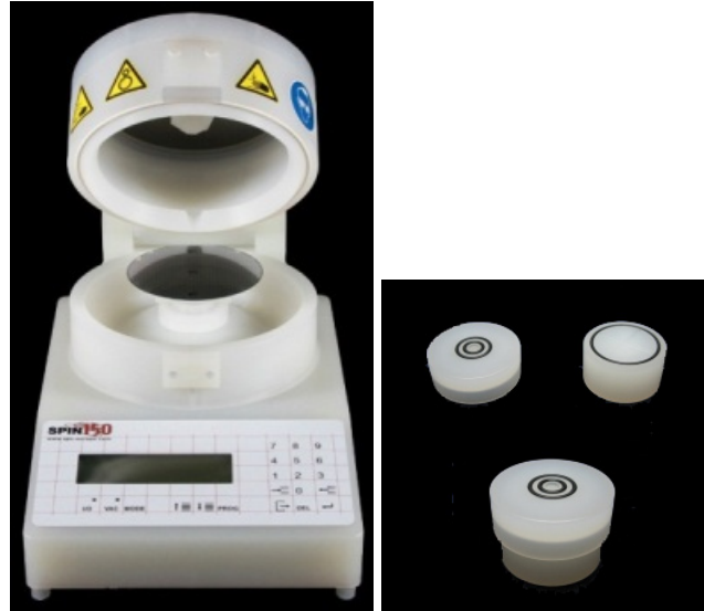
Figure 2.13: (a) SPS Spin 150 wafer spinner and (b) different chucks (substrate holders) used in the spin-coater
