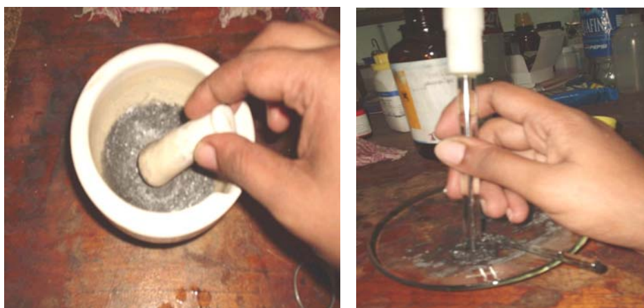
Figure 2.2 Stages involved in the fabrication of a carbon paste sensor
