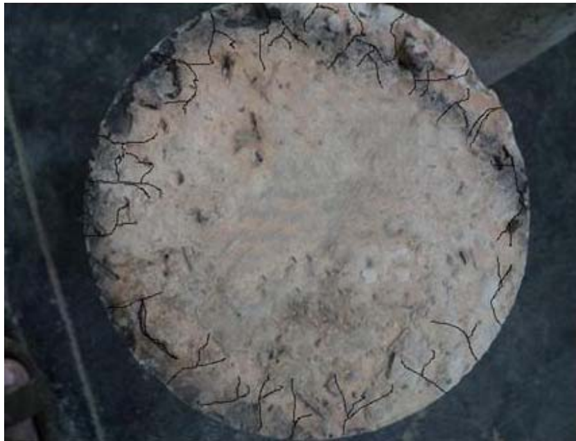
Figure 6.76 Typical crack pattern on LSCCF at 600°C under water cooling
