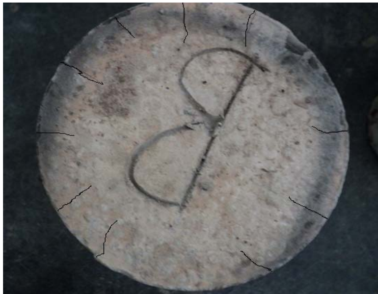
Figure 6.74 Typical crack pattern on LSCCF at 600°C under air cooling
