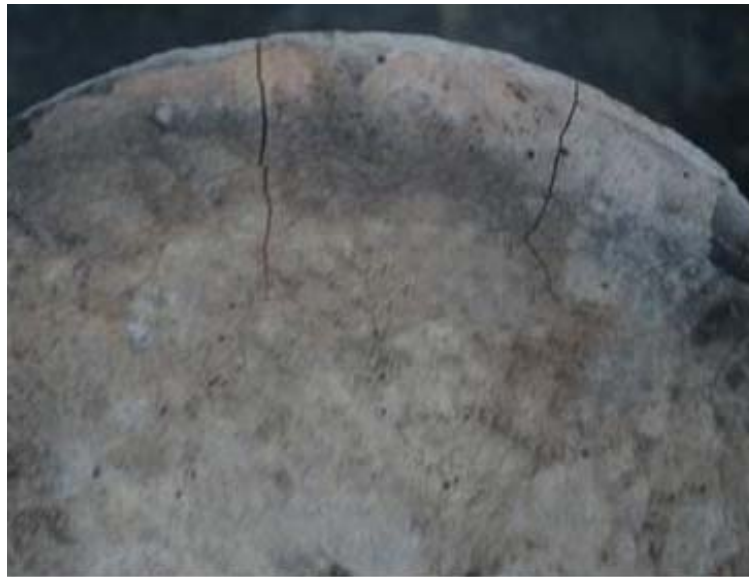
Figure 6.75 Typical crack pattern on LSCCG at 600°C under air cooling-closer view
