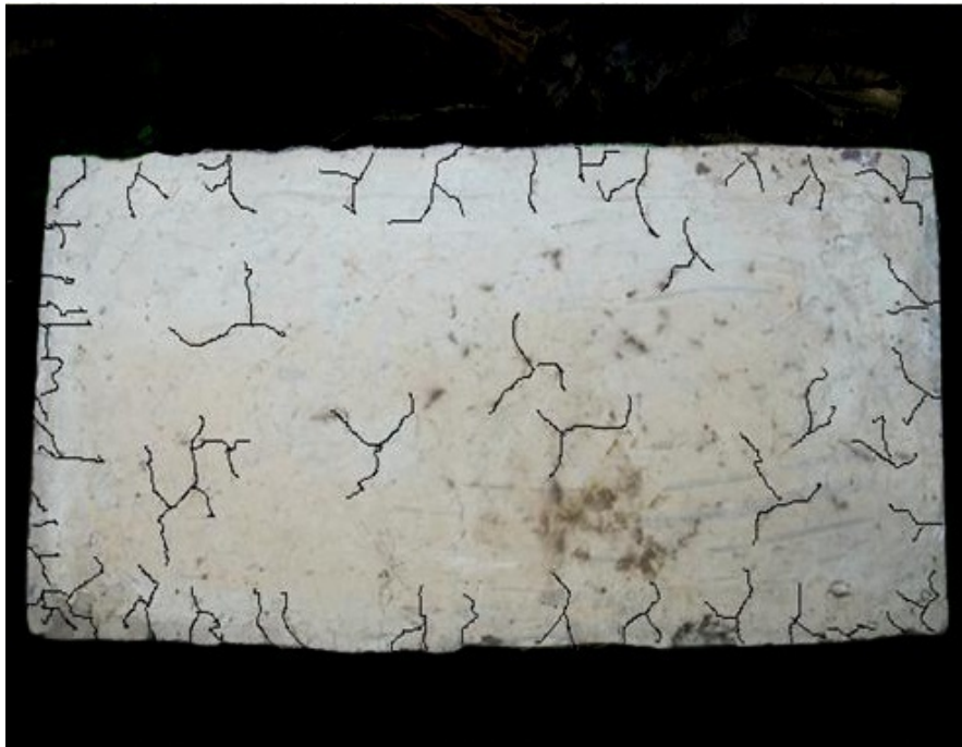
Figure 6.80 Typical crack pattern on specimen heated to 600°C and cooled with sprinkling of water.
