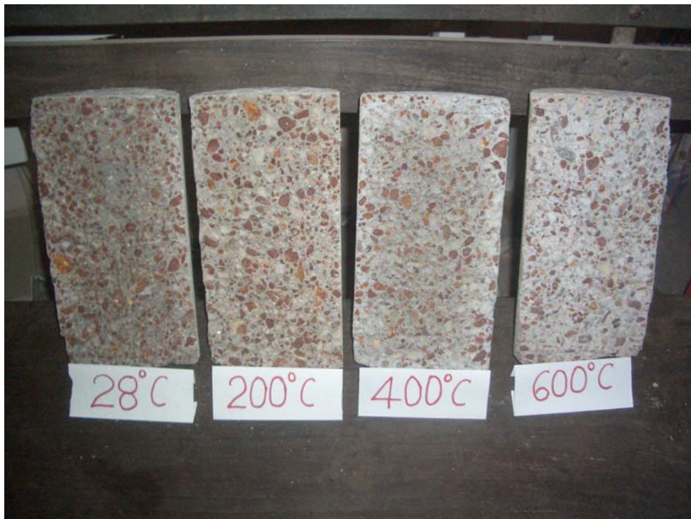
Figure 6.77 Typical colour change of laterised concrete at elevated temperature
