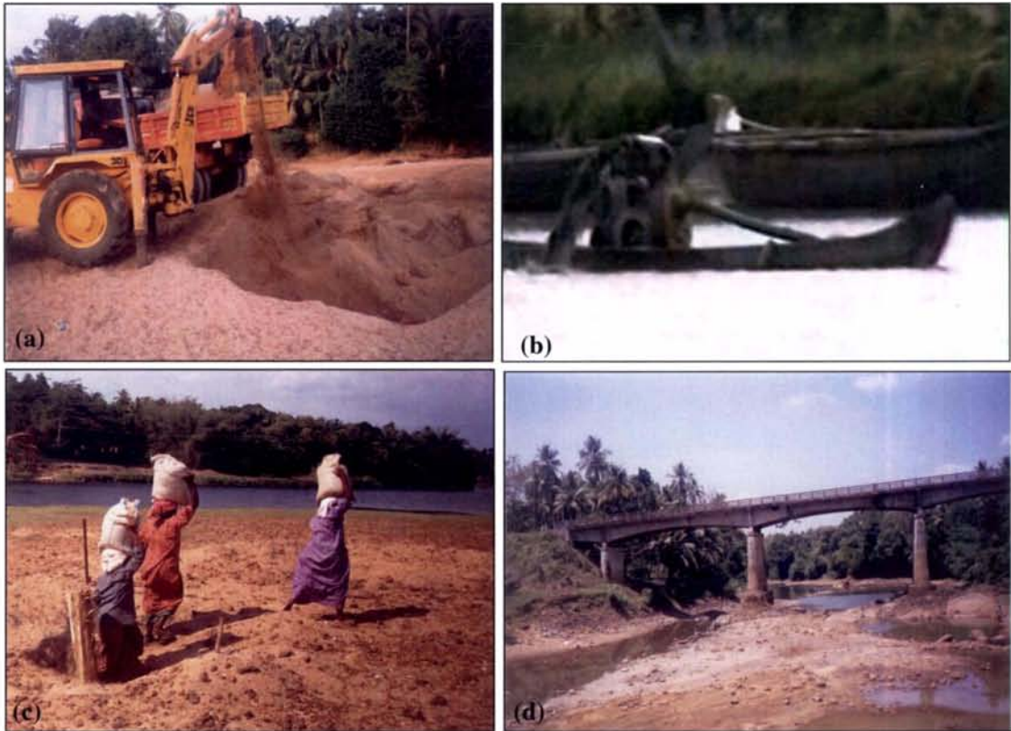
Plate 6.2 Mechanical and manual river sand mining and sand deficient river reach; (a) Dry pit mining of sand using mechanical method; (b) Extraction of sand using high power jet pumps; (c) Bar skimming from the sand bed; (d) A sand deficient reach in Manimala river.
