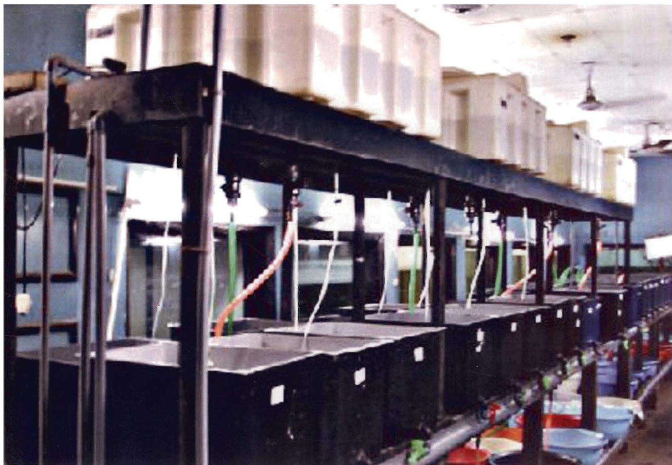
Fig.2.1: Bioassay system used for feeding experiment with F. indicus post larvae for testing immunostimulant property of marine yeasts and beta-1, 3-glucan.
